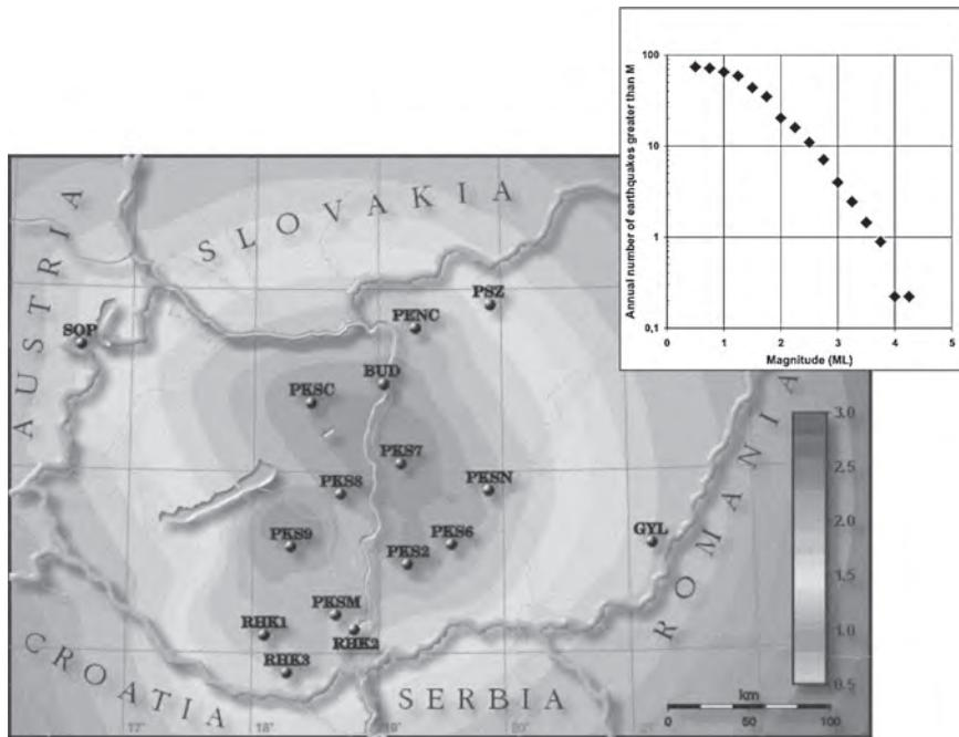
**Figure 4** Predicted and observed detection capability of the Hungarian seismograph network. Contour values are local Richter magnitudes ( $M_L$ ). Criteria for calculation: signal to noise ratio greater than 10 at minimum four stations at average noise conditions. The insert shows the magnitude recurrence curve for Hungary for the recording period 1995–2004
