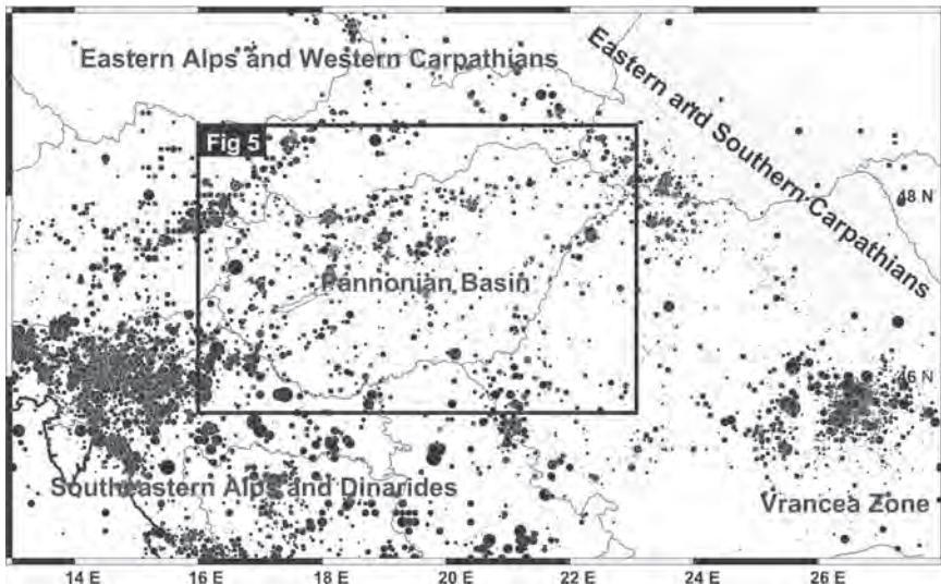
**Figure 1** Seismicity of the Pannonian basin and adjacent area (44.0–50.0N; 13.0–28.0E). The regional earthquake database contains more than 22,000 historical and instrumentally recorded events from AD 456 until 2005 (modified from Tóth et al., 2006). Details on the Pannonian basin seismicity are presented in Figure 5
