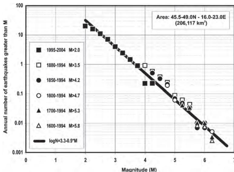
**Figure 6** Magnitude recurrence curve for Pannonian basin earthquakes
