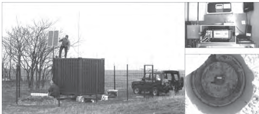
Figure 3 The SP field stations each consist of a three component short period seismometer located in a pit, with a digital recorder and time signal receiver housed nearby in a heat insulated steel container building
